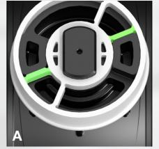
If the valve is over torqued, the topcap is designed to fail before the valve seals, thus preventing a leak to atmosphere. The **safety topcap** can be replaced easily under live conditions.
