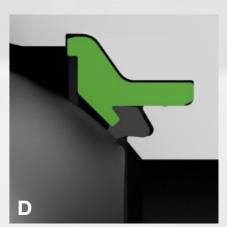
The **seat retainer** design ensures the ball seat is kept in place at all times. This optimal design prevents the ball seat from being dislodged, which guarantees a good functionality throughout the years.
